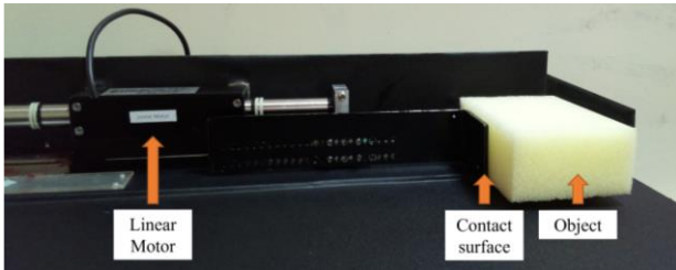
Fig. 7. Experimental setup for the abstraction of haptic information.
